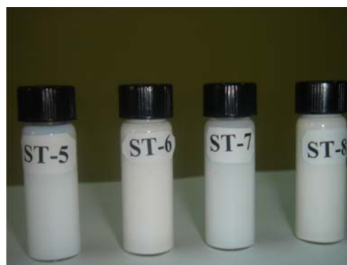
Fig. 4 Colloidal stability of a nanocomposite latex, including 5.3 wt.% Cloisite 30B at different intervals of 30 days (ST-5), 60 days (ST-6), 90 days (ST-7), and 100 days (ST-8)
