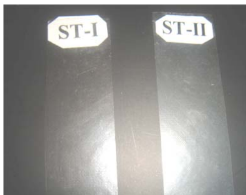
Fig. 6 Films of pure poly(styrene- co -butyl acrylate) (ST-I) and poly(styrene- co -butyl acrylate)–Cloisite 30B nanocomposite, including 5.3 wt.% Cloisite 30B (ST-II)
